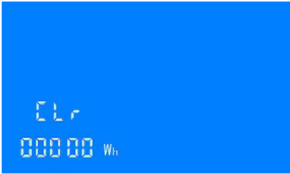
Figure 9 clear the energy interface
